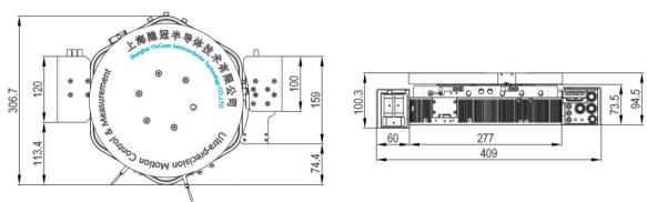
\*Interface dimensions from MZT90 in the middle of vertical stroke
